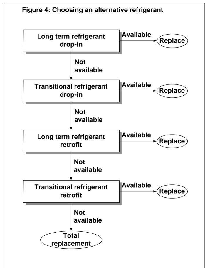
Applying the logic of Figure 4 to the table of R502 alternatives in Figure 5 gives the following results:
