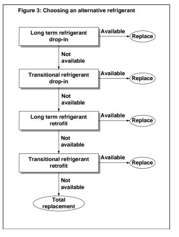
Applying the logic of Figure 3 to the table of R22 alternatives in Figure 4:
